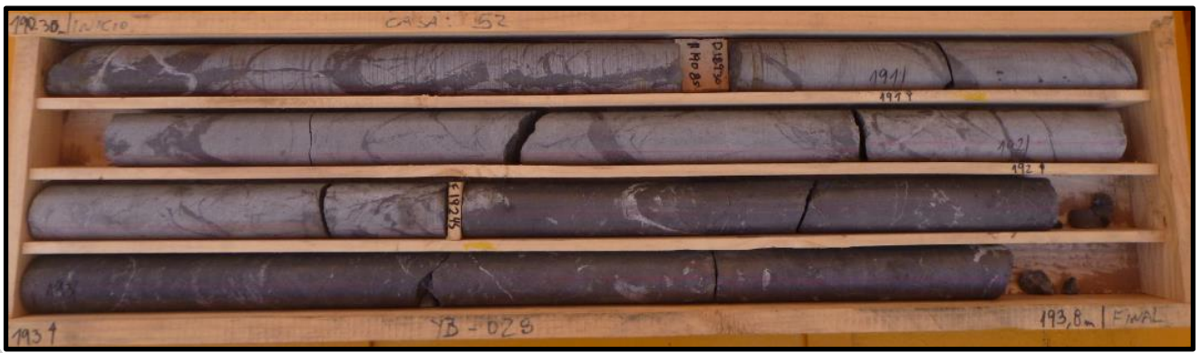
Figure 4 - Core tray 52 from diamond drill hole YB028 showing typical high grade magnetite mineralisation – interval 190.3m to 193.8m shown
