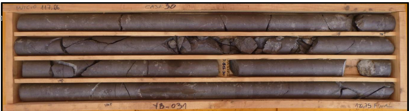
Figure 3 – Core tray 30 from diamond drill hole YB031 showing typical high grade magnetite mineralisation – interval 117.06m to 120.75m shown
