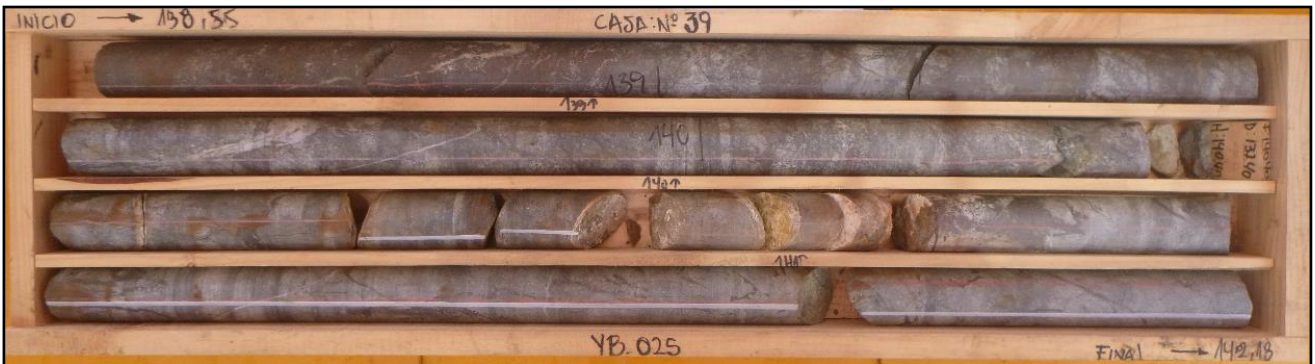
Figure 2 - Core tray 39 from diamond drill hole YB025 showing typical high grade magnetite mineralisation – interval 138.5m to 142.2m shown
