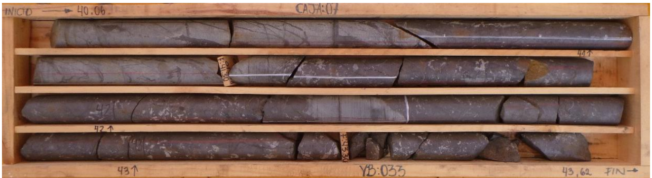
Figure 5 - Core tray 07 from diamond drill hole YB033 showing high grade magnetite mineralisation – interval 40.1m to 43.6m shown
