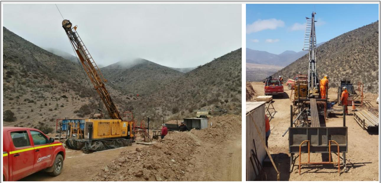
Figure 1 – Diamond drill rig in position at ES001 ready to test copper target anomaly
